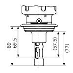
SensoGate® WA 131 H Process adaptation for Varivent from DN 65, short immersion depth
