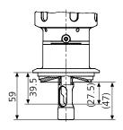
SensoGate® WA 131 H Process adaptation for Varivent from DN 80, long immersion depth
