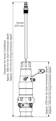
SensoGate® WA 131 H Process adaptation for Varivent DN 50, short immersion depth
