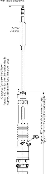
Installation dimensions for SensoGate® WA 131 H for sensors with gel electrolyte
