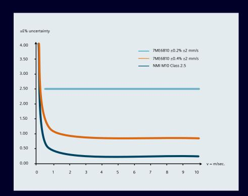
A calibration certificate is supplied with every water meter, and all calibration data is stored in the instrument.
